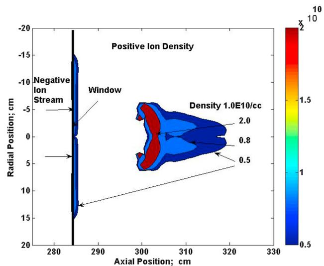
**Figure 4.** Positive ion density at the end of the second pulse.
