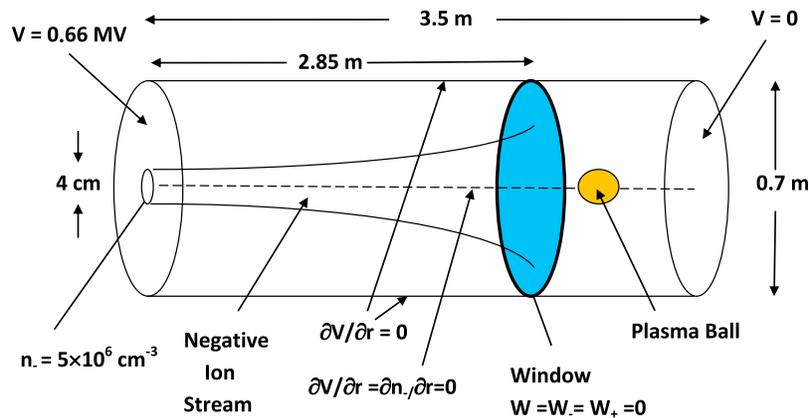
**Figure 1.** Calculation domain and boundary conditions.
