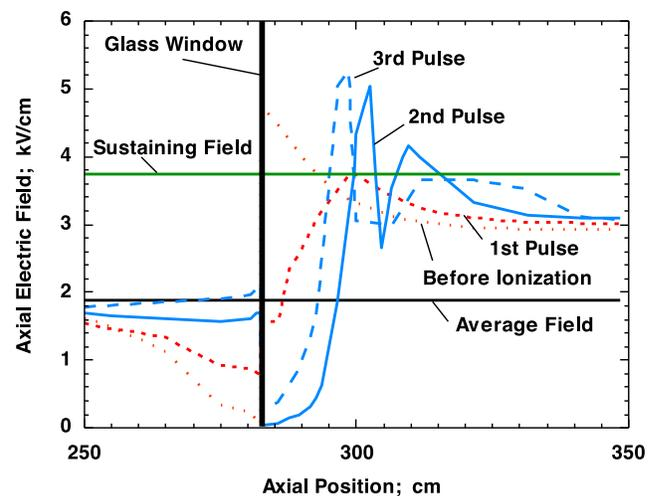
**Figure 2.** Axial field distributions at various discharge times.
